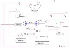
Fig.3 Architecture Of BFD Multiplier
